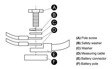
**IMPORTANT:** Attach the cable as close as possible to the battery poles, but above the battery connectors.
