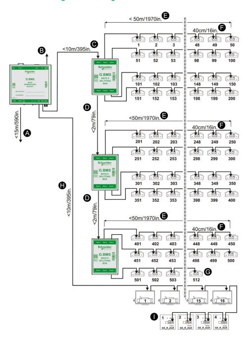
**IMPORTANT:** The maximum distance between the last module or device and the webmanager is always 60 m (196 ft), **(C)** + **(E)**, **(C)** + **(D)** + **(E)** or **(C)** + **((D)** \* 2) + **(E)**, depending on the number of splitting boxes. A splitting box does not increase the maximum distance.
