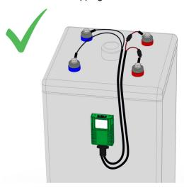
Do not place the G.BMS modules on any cooling ribs or plugs.
