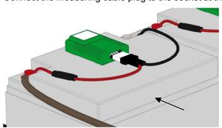
**NOTE:** The measuring cable is equipped with a mechanical protection against accidental polarity reversal.
