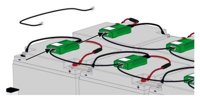
**NOTE:** Do not use the module closest to the webmanager or splitting box to connect the rows.
