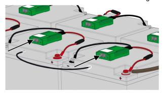
2. If applicable, connect the bus cables between the modules at the end of the rows.
