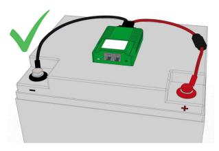
If there is not enough space on the top of the battery, place the G.BMS module on the front panel of the battery.
