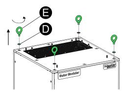
Only for systems without a rain roof and any lifting eye locations outside the rain roof: Attach and tighten the cabinet roof screws and washers.
