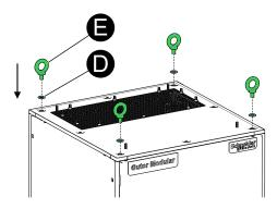
3. Tighten the lifting eye bolts (E) to a torque of 10 Nm (88.5 lbf-in).
