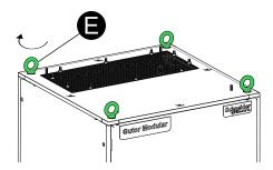
4. Make sure that lifting eye bolts (E) are attached to all lifting locations.
