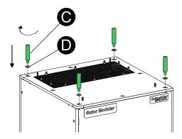
2. Place the roof (B) on top of the distance bolts.
