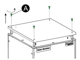
3. Lift off and remove the roof (B).
